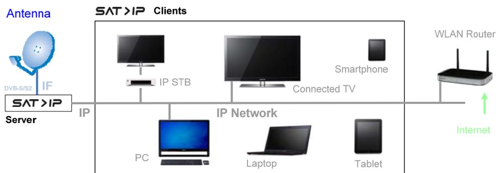
In order to realise this step change in satellite reception, a new manufacturer independent protocol was designed which allows various SAT>IP client devices to communicate with SAT>IP servers.
