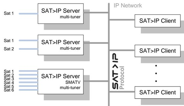
SAT>IP clients talk to SAT>IP servers using the SAT>IP protocol.
